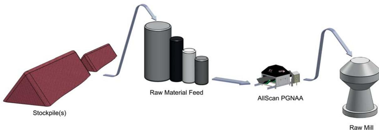
In both applications the data from the **AllScan** is seamlessly transferred to the plant control system and is typically interfaced to 3rd party QC optimization software to improve quarry operations, stockpiling and raw mix proportioning.
